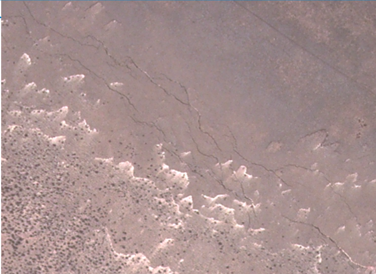
Ground rupture induced by the earthquake in the remote sensing image
